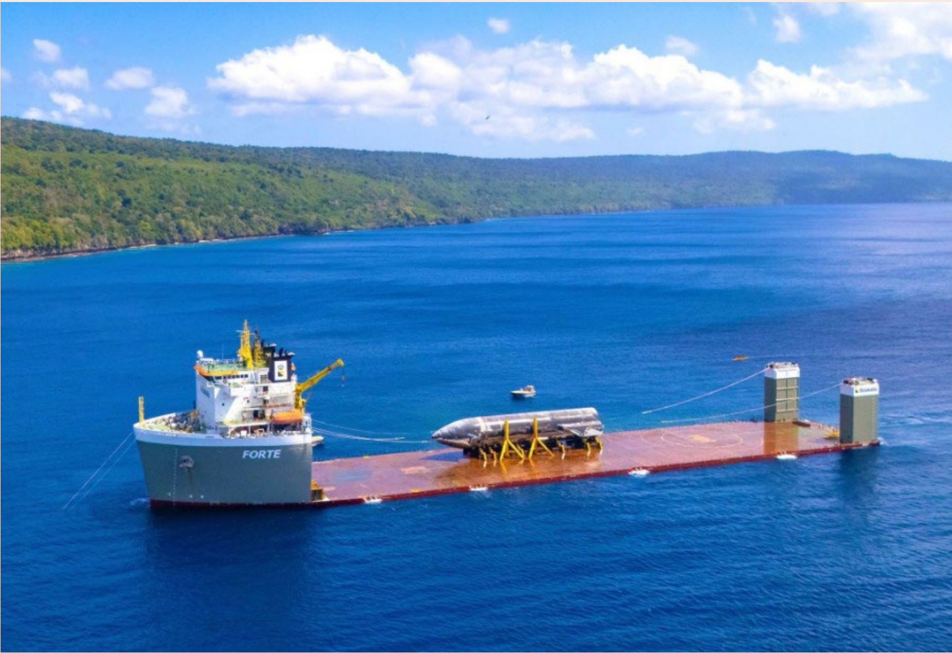
Space X Ship 40 loaded on Semi-submersible vessel Forte. Photo credit: © Chris Bray Photography
