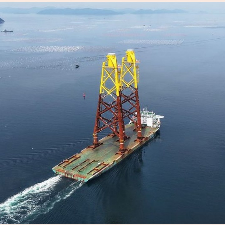
SK oceanplant ships two jacket foundations. (Image source: SK oceanplant via LinkedIn)
