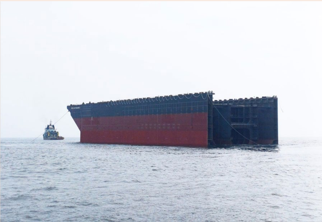
Forward Section of MODEC's Next Generation Hull for FPSO Gato do Mato (Image source: Modect)
