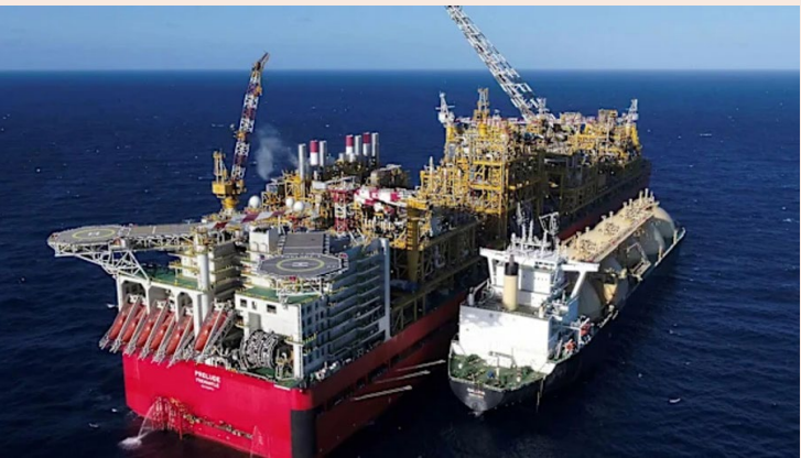
Shell's Prelude FLNG facility operates offshore from Western Australia without a pipeline connection to the mainland.
