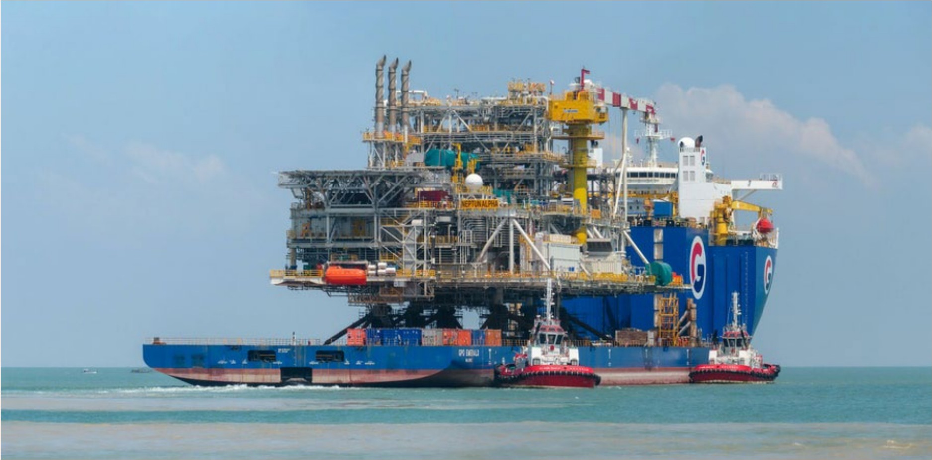
GPO Emerald loaded with Neptun Deep topside (Image courtesy of GPO Heavylift)
