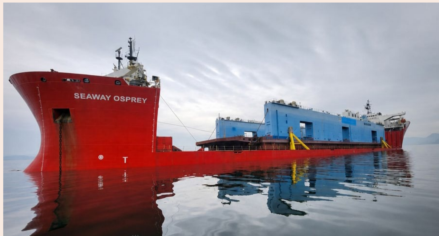
Seaway Osprey loads a 120 x 34 m floating dock in Geoje, South Korea.
