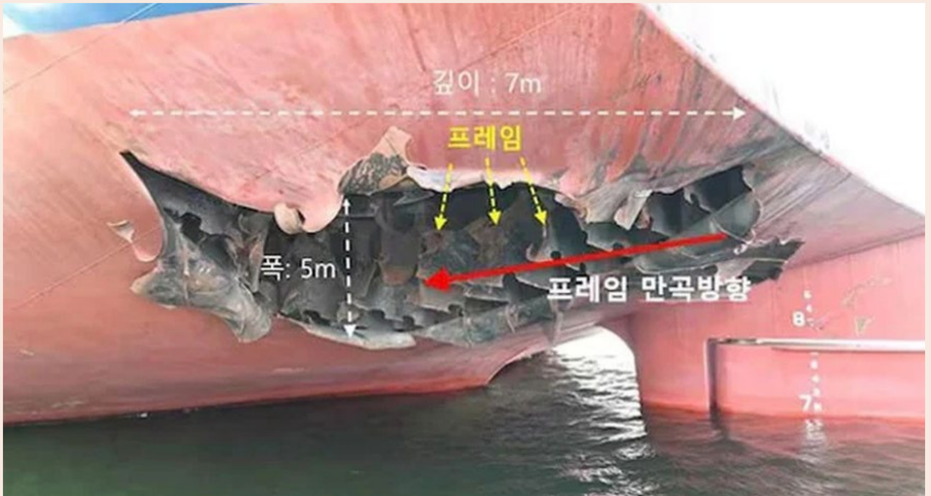
Hull damage identified on HMM Namu following the PersianGulf incident. (Image source: Foreign Ministry)
