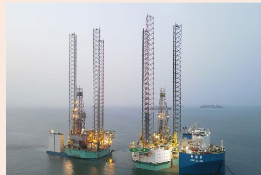
Heavy lift vessel GPO Sapphire transporting Shelf Drilling Victory and High Island II in April 2025. (Image source: TLC)
