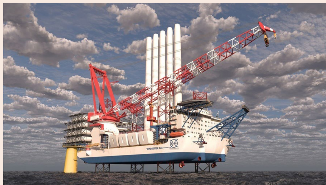
WindSetter 146 class Wind Turbine Installation Vessel
