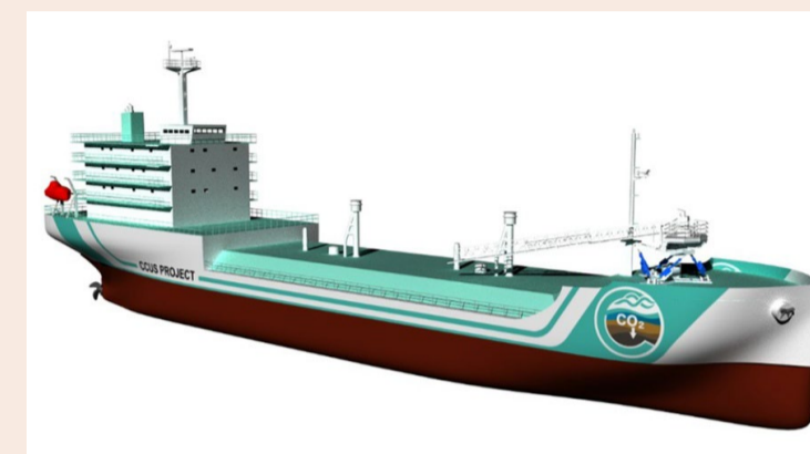
Illustration of Japan's CO2 carrier concept with gangways for connection at the storage site. (Image source: SSS)
