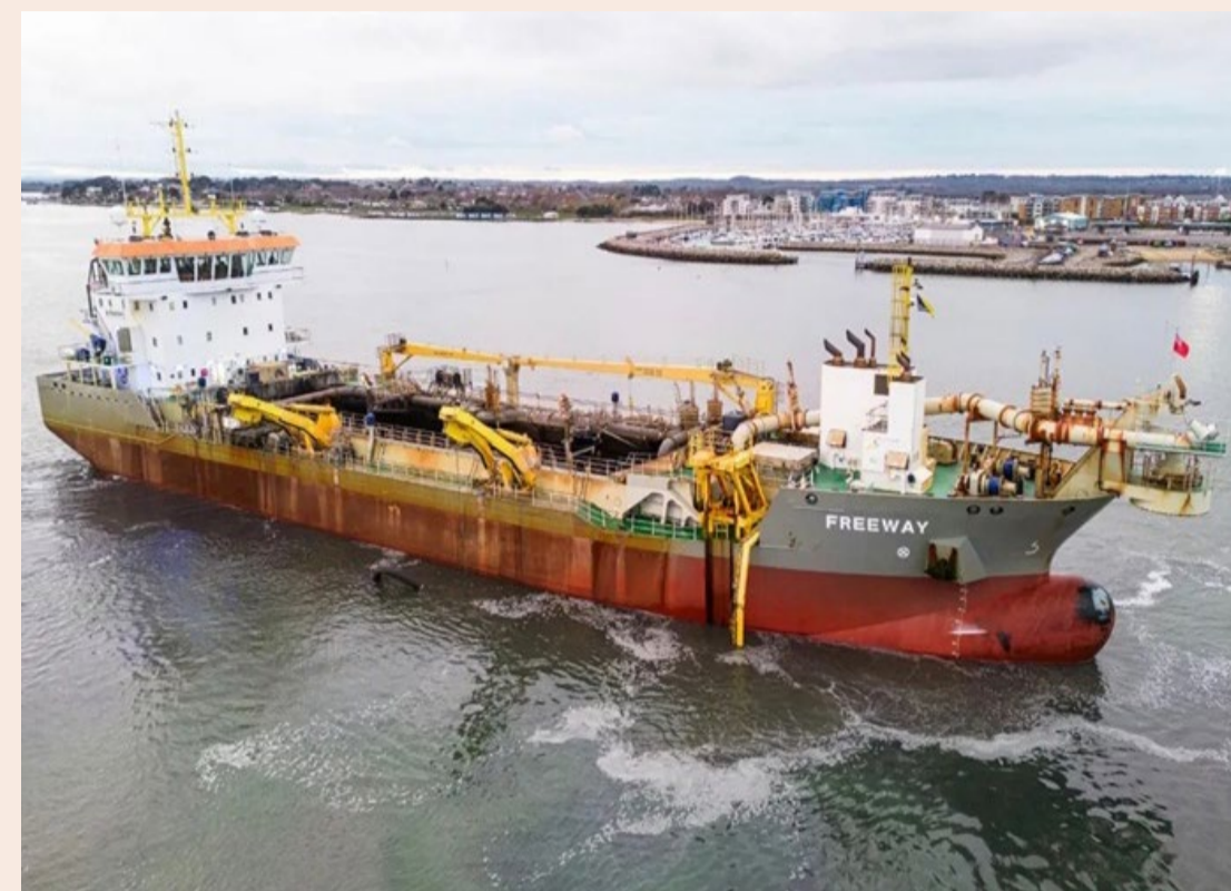
Boskalis Westminster Ltd's Freeway trailing suction hopper dredger (Source: Port of Aberdeen)
