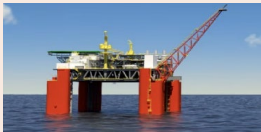
Illustration of Kaskida's semisubmersible production unit, designed for up to 80,000 BOPD. Source: Exmar
